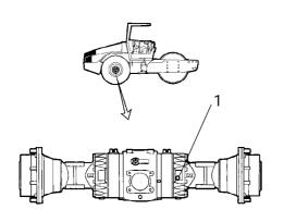
Fig. Level check - differential housing 1. Level/Filler plug
