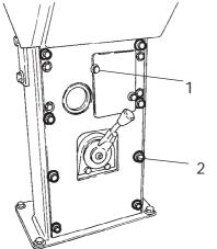
Fig. Instrument column 1. Screws for fusebox cover (2) 2. Screws for column cover(12)
