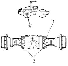
Fig. Rear axle 1. Level/Filler plug 2. Drain plugs
