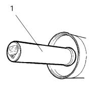
Fig. Air filter 1. Backup filter
