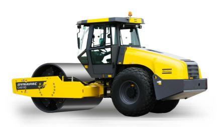
The Dynapac CA510 is a roller in the 18-ton class. CA510 is available in D (smooth drum) and PD (padfoot drum) versions. CA510D is intended for the compaction of rockfill. The main area of application for the CA510PD is on cohesive material and weathered stone material.
