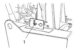
Fig. Engine compartment 1. Master switch
