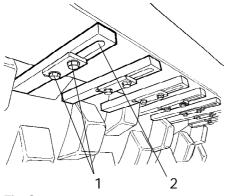
Fig. Scrapers 1. Screws 2. Scraper teeth (x18)
