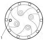
Fig. Level check - planetary gear 1. Level/Filler plug
