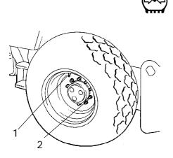
Fig. Wheels 1. Air valve 2. Wheel nut
