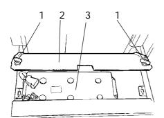
Fig. Battery shelf 1. Quick-screws 2. Battery cover 3. Battery
