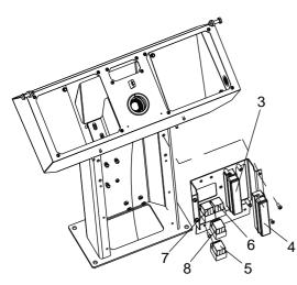
Fig. Instrument panel with fuses and relays.
