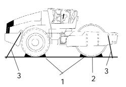
Fig. Transport 1. Chock 2. Block up 3. Lashing wire
