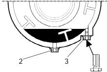
Fig. Drum cartridge 2. Drain plug 3. Level plug
