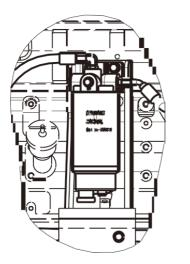
Fig. Engine compartment 1. Fuel prefilter
