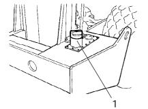
Fig. Fuel tank 1. Filler pipe
