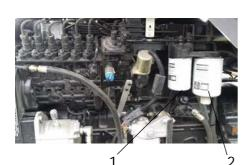
Fig. Oil level check - drum gearbox
