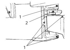
Fig. Steering hitch right side 1. Lubricating nipples articulation (x4) 2. Lubricating nipple cylinder mount (x1)
