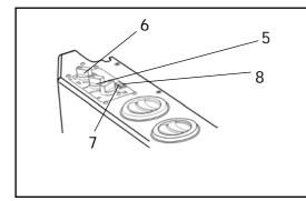
Fig. Cab, right side. Heater (Optional) 5. Control, temperature 6. Control, circulation, 7. Control, fan 8. Switch, AC (Optional)
