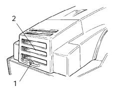
Fig. Engine hood 1. Hood lock 2. Protective grille
