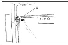
Fig. Cab roof, rear 4. Hammer for emergency escape
