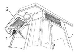
Fig. Air conditioning 1. Refrigerant hoses
