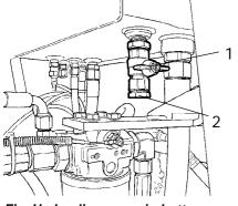
Fig. Hydraulic reservoir, bottom 1. Drainage tap 2. Plug
