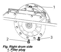
Wipe clean the filler plug (1) and level plug (3). Unscrew the filler plug (1).
