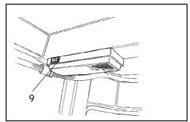
Fig. Cab, rear 9. Switch, cab lighting (Optional)
