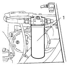
Fig. Engine compartment 1. Hydraulic fluid filter (x1)
