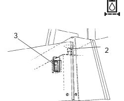
Fig. Hydraulic reservoir 2. Filler cap/Air filter 3. Sight glass
