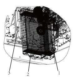
Fig. Radiator 1. Intercooler 2. Coolant radiator
