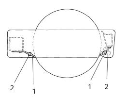
Fig. Scrapers 1. Scraper blade 2. Screws
