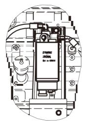
Fig. Engine compartment 1. Fuel prefilter
