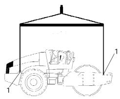
Fig. Roller prepared for lifting 1. Hoisting plate
