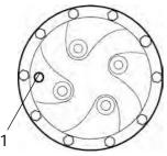
Fig. Planetary gear/filling position 1. Plug
