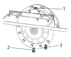
Fig. Right drum side 1. Filler plug 2. Drain plug
