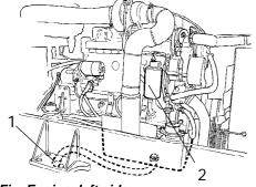
Fig. Engine, left side 1. Drainage plug 2. Oil filter
