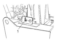
Fig. Engine compartment 1. Master switch
