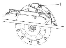
Fig. Drum 1. Ventilation screw
