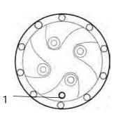
Fig. Planetary gear/drainage position 1. Plug
